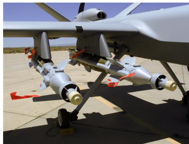
MQ-9 Reaper with GBU-38 JDAMs loaded.
