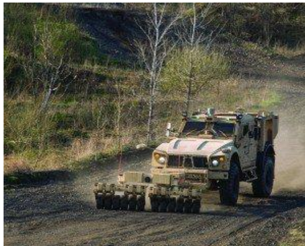
The unmanned TerraMax M-ATV with its mine roller.
