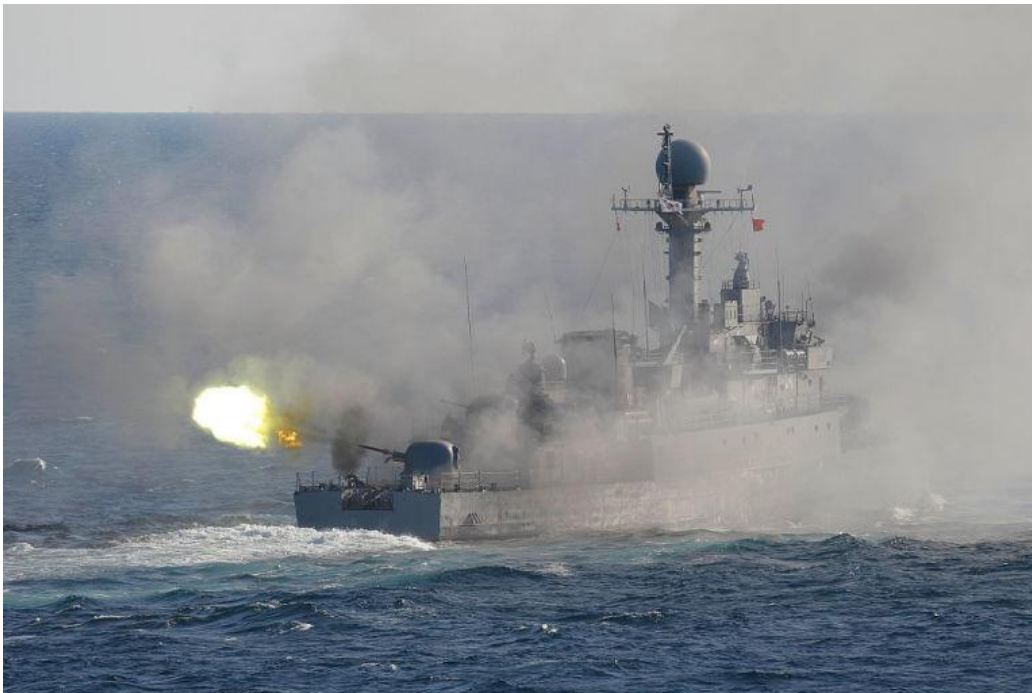
Pohang-class corvette firing its stern mounted 76-millimeter gun during a fleet review, 2015.
